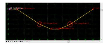
Constrain the hinge points. Note for the first hinge point, the Constraint 2 **Vertical** value is arbitrary. (Part I of the delta training).
