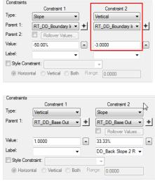
Attach the new customized ditch component to the end conditions of your template and establish the required "Parent-to-Child" relationship (Part I of the delta training).
