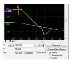
However, if we choose the first hinge point as Point Controls with a vertical offset of 1' then the desired effect is achieved. Remember there is a 1' vertical difference between the bottom ditch base and hinge point 1 (design assumption fixed 3:1 slopes).
